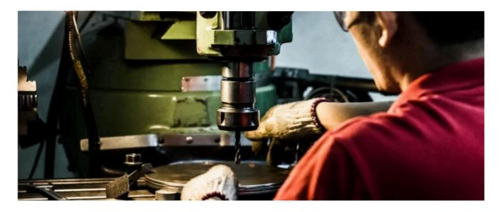
The machinist manually controls the machine, manipulating levers and handles to move the cutting tool against the workpiece. They rely on their experience to determine factors like cutting speed, feed rate, and depth of cut. As the cutting tool comes into contact with the workpiece, it removes material through shearing. The machinist continuously observes the process, adjusting to maintain proper cutting conditions and achieve the desired shape.
